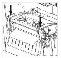
**5.** Move the media sensor by adjusting the media sensor position adjustment knob, make sure the gap or black mark sensor is at the location where media gap/black mark will pass through for sensing. Adjust the label guide to fix the media position.
