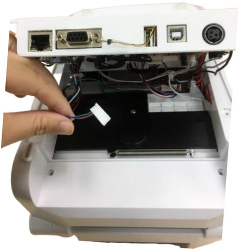
5. After opening, pull out the wire just put into the hole and insert it into the wafer 1x7P P1.25 connector on the main board
