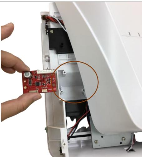
5. After opening, insert this cutter board and lock the cutter board with two screws
