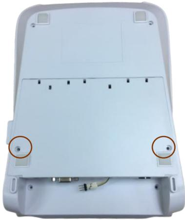
4. Turn the printer upside down, remove the two screws located on the bottom cover, and open the bottom cover
