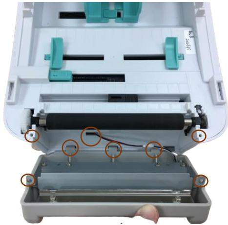
2. Align the cutter with the tenon, and place the wire of the cutter into the hole
